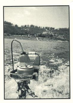
Tom Lockwood worked with George Kent honing cylinders and reassembling the 1948 Mercury, 3.6 hp KE3 above. They worked so hard that when George brought it to the meet they were really anxious to get it running, so anxious that they duck tapped a plastic gas can on it, line and all, and off it went. Tom Lockwood says, "If you bring your oars, your motor will always start." "There is truth in that, says George, I did and they ran beautifully."
